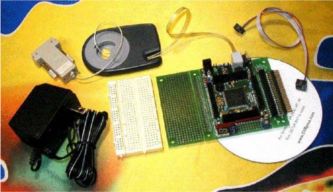
Above is a picture of the MiniDragon+ Development board from [www.evbplus.com](http://www.evbplus.com). This is the board that is used for the Lotus project and it contains a MC9S12DP256. This controller has 256KB of Flash, 12KB of SRAM, 4KB of EEPROM and is internally clocked at 24MHz.
