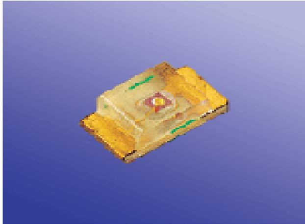
The LEDs are 0805 package surface mount devices that are soldered to the Custom Interface Board. There is one Blue LED that is a power led that is tied to the power rail that turns on whenever the power is applied to Lotus. There are two Blue LEDs, two Red LEDs, and four Green LEDs. The Custom Interface Board contains eight LEDs that are indirectly tied to the eight PWM outputs of the HCS12. This will give the LEDs the ability to have a “fade” effect (LEDs can be more than just ON or OFF).
